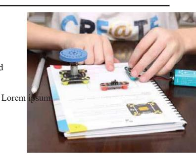
magnetic components that snaps right into your circuit, which are buzzer, eight pin, LED, button, etc. without any hassle of gluing or soldering. At a conventional low cost and high quality, learning is just getting better.
