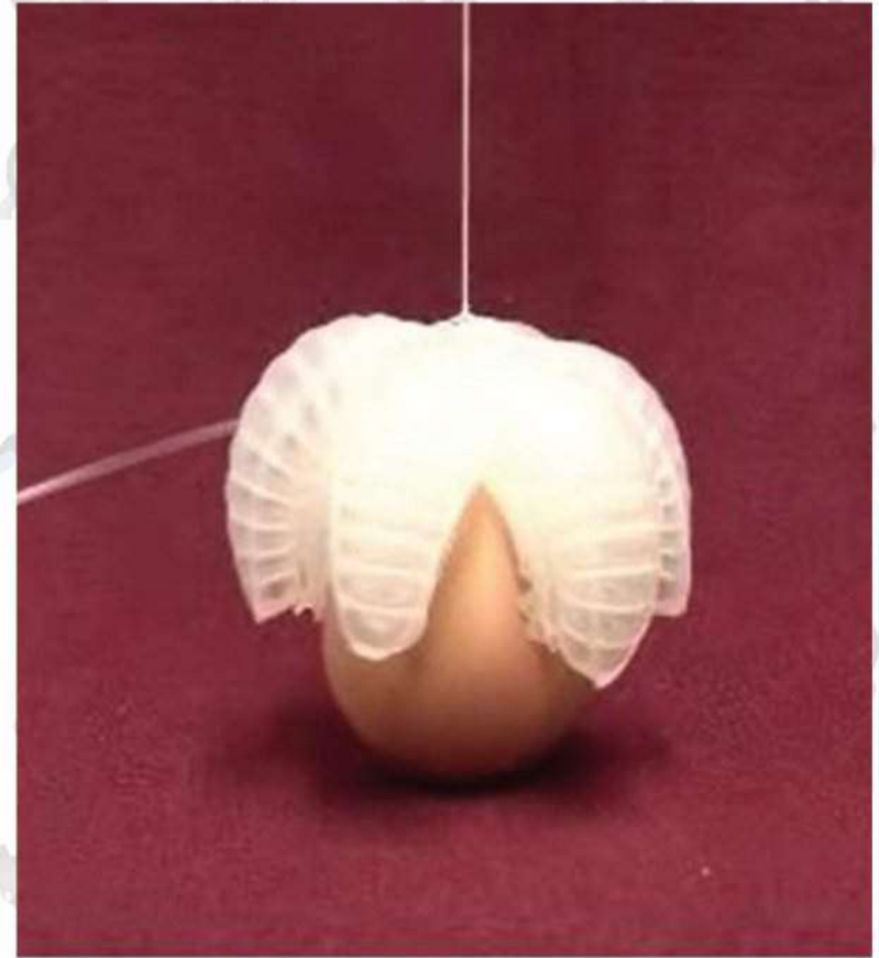
FIG. Soft Gripper based on PneuNets Actuators to lift egg. Developed at HARVARD
