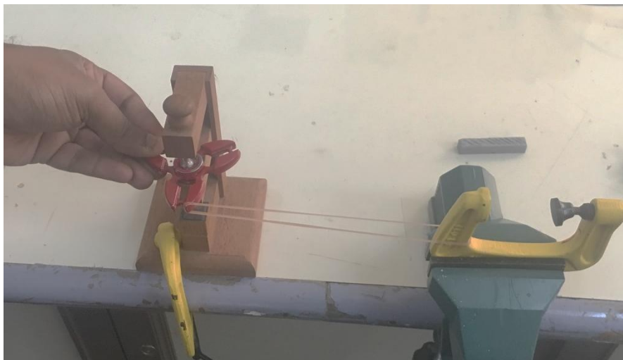
Fig 2: Setup to provide uniform input to the spinner. Students should ensure that a rubber band can be attached to the spinner.
